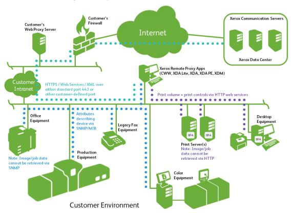
Figure 3.2.1 System Components & Data Flows of the Remote Proxy App-based Model
