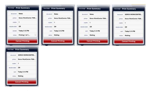
On the Xerox<sup>®</sup> device, select the **Job Status** button. Observe the device Print Queue (Active Jobs) and notice that only the first job from that Apple iOS device is visible. It is the only job that has been sent to the Xerox<sup>®</sup> device from that Apple iOS device. Once this job completes, the next job queued on the Apple iOS device will be sent to the Xerox<sup>®</sup> device.
